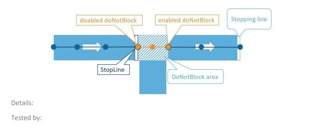
A SegmentAttributeXY of value 'doNotBlock' shall be present in the 'enabled' list at the first node of the lane that shall not be blocked by a vehicle in case of a queue in front of the traffic light.
