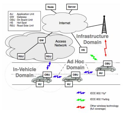
Figure 3 Draft reference architecture
