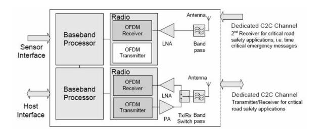
Figure 15 Dual receiver concept
