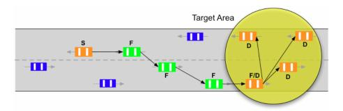
Figure 19 Geographically-scoped broadcast with packet transport towards the target area
