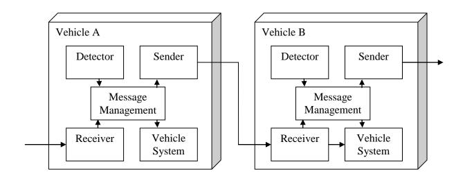
Figure 11 Application instances for Vehicle 2 Vehicle Decentralized Environmental Notification
