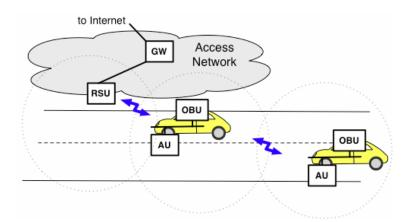
Figure 7 A RSU provides Internet access
