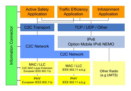
Figure 8 Protocol architecture of the C2C Communication System
