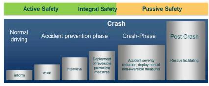
Figure 7: Phases of the vehicular safety system (Ref: C2C-CC)
