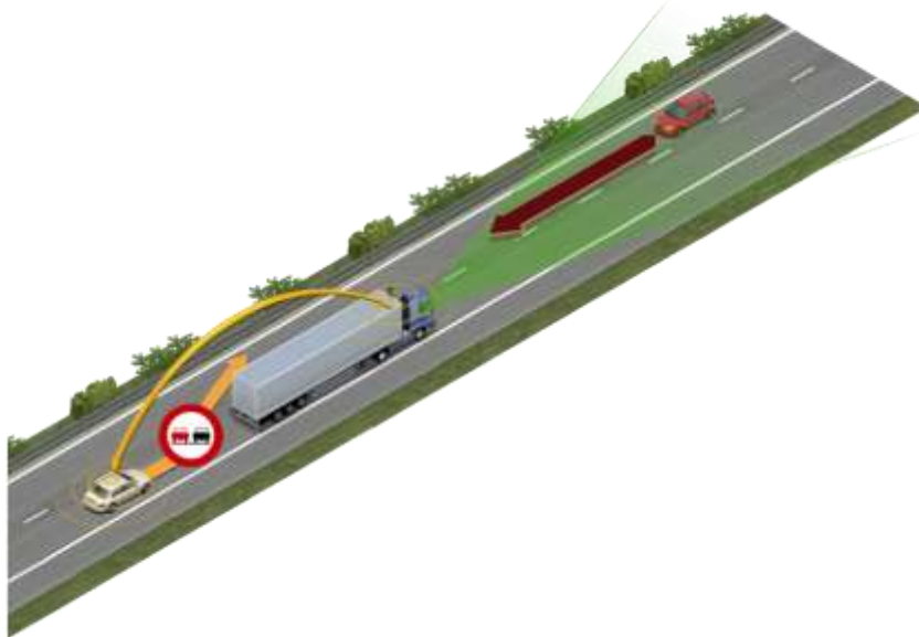
Figure 3-6: Sample scenario of the cooperative overtaking on rural roads use case. The truck sends a CPM (yellow arrow) with information on the detected red car.
