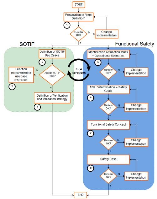
Figure 16 Evaluation process determining the SOFIT and Functional Safety requirements (ENSEMBLE)
