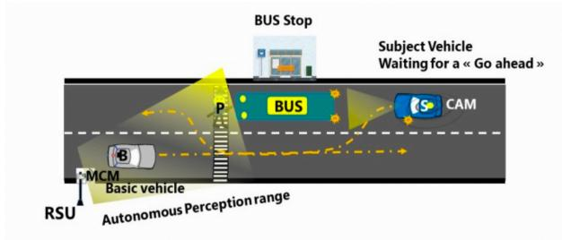
Figure 10: LCA-B Situation description (ETSI TR 103 578).
