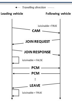
Figure 8: PCM information exchange example (ENSEMBLE)
