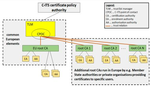
Figure 14: Certificate Trust Model Architecture
