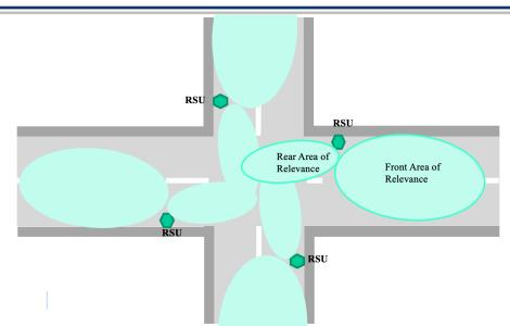
Figure 13: RSU Placement and Message transmission patterns example
