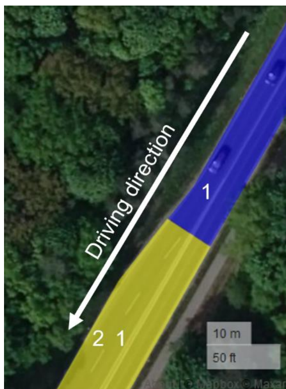
Figure 44: ADASIS-road segments for the scenario in clause 3.4 with the expected ETSI LanePositions. (Source: created using https://geojson.io © Mapbox (see: https://www.mapbox.com/about/maps/ ) © Maxar (see: https://www.maxar.com/ ))
