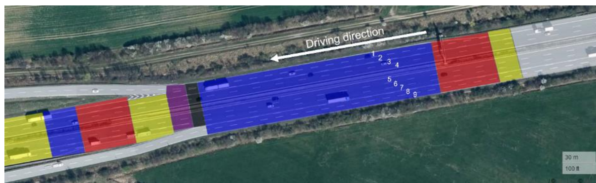
Figure 26: Coloured overlay of the A2 showing the road segmentation according to the ADASIS rules. The general driving direction and lane numbering for one segmented are added. (Source: created using https://geojson.io © Mapbox (see: https://www.mapbox.com/about/maps/ ) © Maxar (see: https://www.maxar.com/ ))
