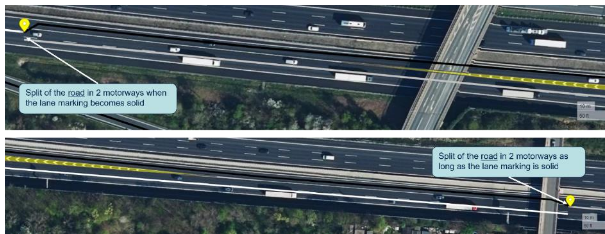
Figure 25: Scenario in clause 3.2 with yellow markers for the start and end points of road links and the different road links in between in white and black. The restricted area between the carriageways is highlighted in yellow. (Source: created using https://geojson.io © Mapbox (see: https://www.mapbox.com/about/maps/ ) © Maxar (see: https://www.maxar.com/ ))
