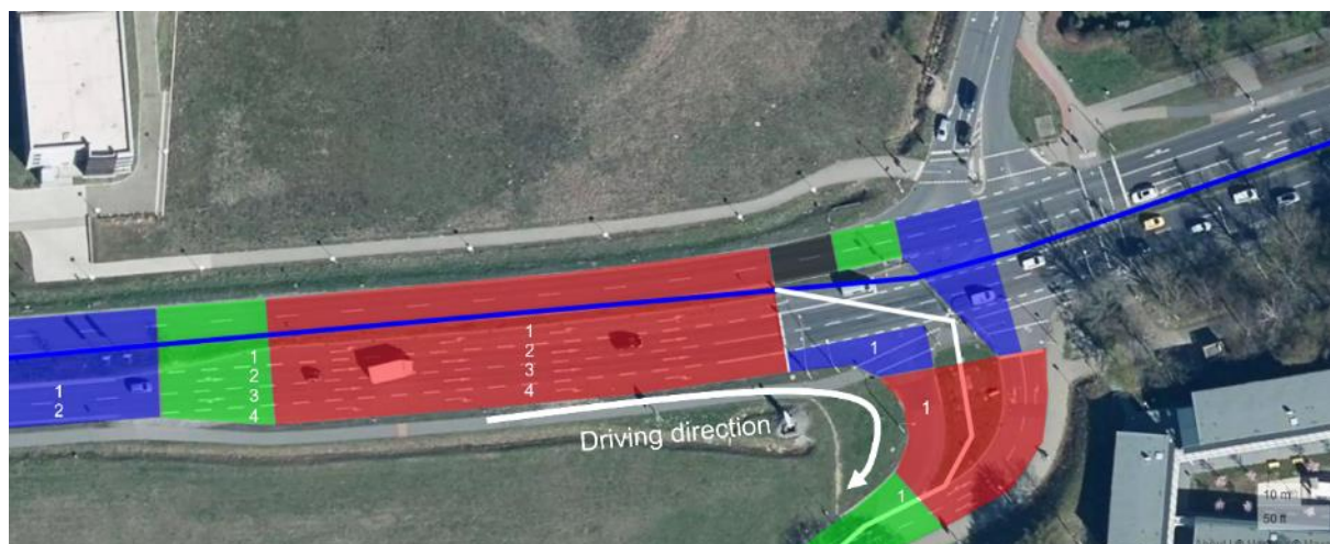
Figure 51: ADASIS-road segments for the scenario in clause 3.7 with the expected ETSI LanePositions for vehicles turning right. The solid line white line diverging from the blue one is the more general path to follow. (Source: created using https://geojson.io © Mapbox (see: https://www.mapbox.com/about/maps/ ) © Maxar (see: https://www.maxar.com/ ))
