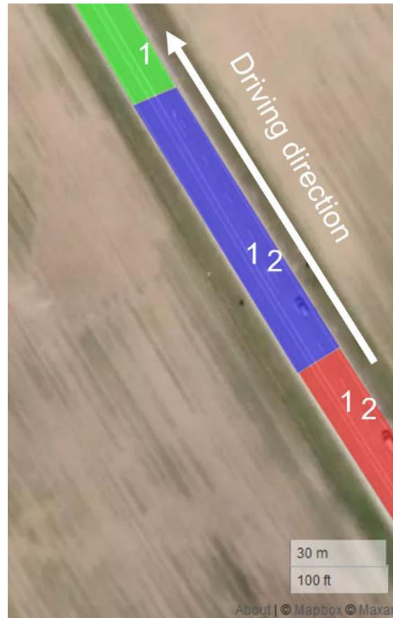
Figure 45: ADASIS-road segments for the scenario in clause 3.5 with the expected ETSI LanePositions. (Source: created using https://geojson.io © Mapbox (see: https://www.mapbox.com/about/maps/ ) © Maxar (see: https://www.maxar.com/ ))
