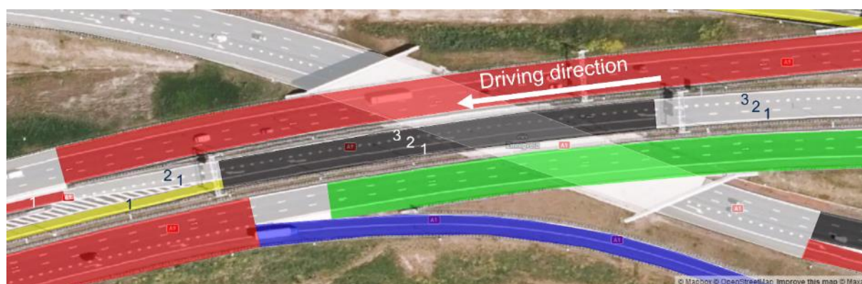
Figure 41: ADASIS-road segments for the central crossing of scenario in clause 3.3 (where the motorways cross each other) with the expected ETSI LanePositions. (Source: created using https://geojson.io © Mapbox (see: https://www.mapbox.com/about/maps/ ) © Maxar (see: https://www.maxar.com/ ))
