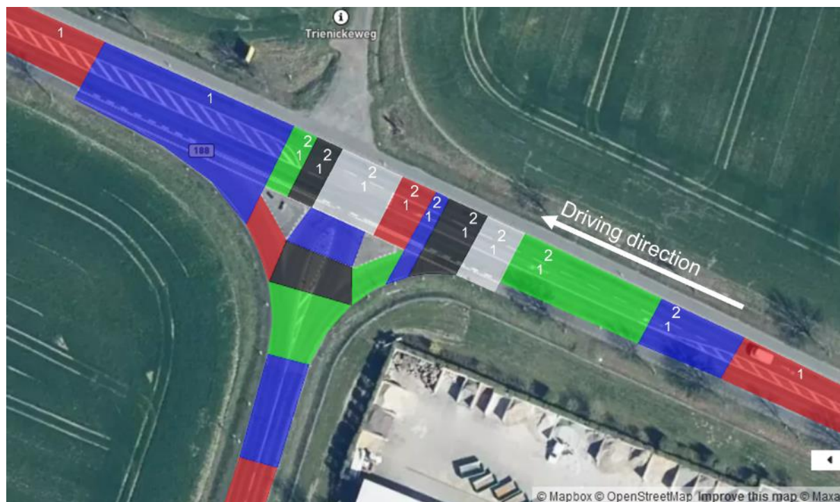
Figure 62: ADASIS-road segments for the scenario in clause 3.12 with the expected ETSI LanePositions for vehicles crossing the intersection straight. (Source: created using https://geojson.io © Mapbox (see: https://www.mapbox.com/about/maps/ ) © Maxar (see: https://www.maxar.com/ ))
