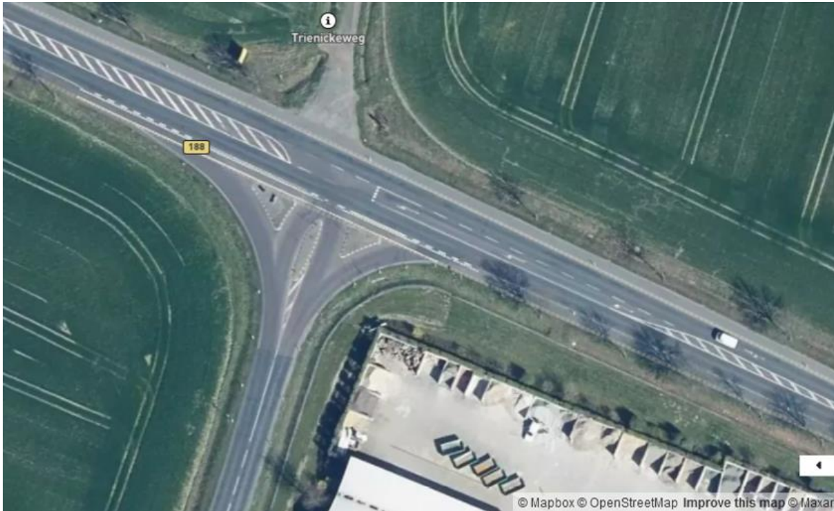
Figure 20: Rural intersection in a T-shape with bicycle lanes beside the road and in the conflict zone. (Source: created using https://geojson.io © Mapbox (see: https://www.mapbox.com/about/maps/ ) © Maxar (see: https://www.maxar.com/ ))
