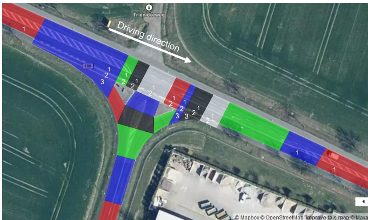
Figure 59: ADASIS-road segments for the scenario in clause 3.12 with the expected ETSI LanePositions for vehicles crossing the intersection straight. (Source: created using https://geojson.io © Mapbox (see: https://www.mapbox.com/about/maps/ ) © Maxar (see: https://www.maxar.com/ ))
