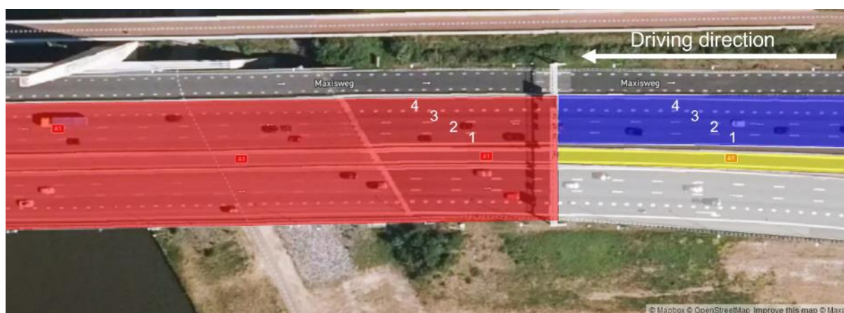
Figure 39: ADASIS-road segments for the 'Muiderbrug' of scenario in clause 3.3 (where the exit lane starts) with the expected ETSI LanePositions. (Source: created using https://geojson.io © Mapbox (see: https://www.mapbox.com/about/maps/ ) © Maxar (see: https://www.maxar.com/ ))
