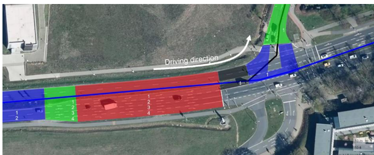
Figure 52: ADASIS-road segments for the scenario in clause 3.7 with the expected ETSI LanePositions for vehicles turning left. The solid line white line diverging from the blue one is the more general path to follow. (Source: created using https://geojson.io © Mapbox (see: https://www.mapbox.com/about/maps/ ) © Maxar (see: https://www.maxar.com/ ))
