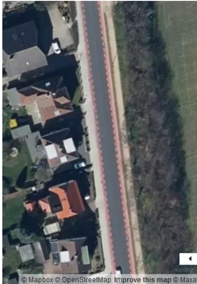
Figure 14: The “Messeweg”, a 2-1 road in Brunswick with a central, shared lane for both traffic directions and a bicycle lane on both sides. (Source: created using https://geojson.io © Mapbox (see: https://www.mapbox.com/about/maps/ ) © Maxar (see: https://www.maxar.com/ ))
