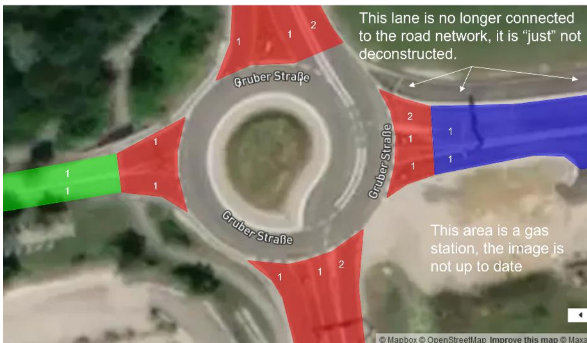
Figure 55: ADASIS-road segments for the ingress / egress roads for the scenario in clause 3.10 with the expected ETSI LanePositions. (Source: created using https://geojson.io © Mapbox (see: https://www.mapbox.com/about/maps/ ) © Maxar (see: https://www.maxar.com/ ))
