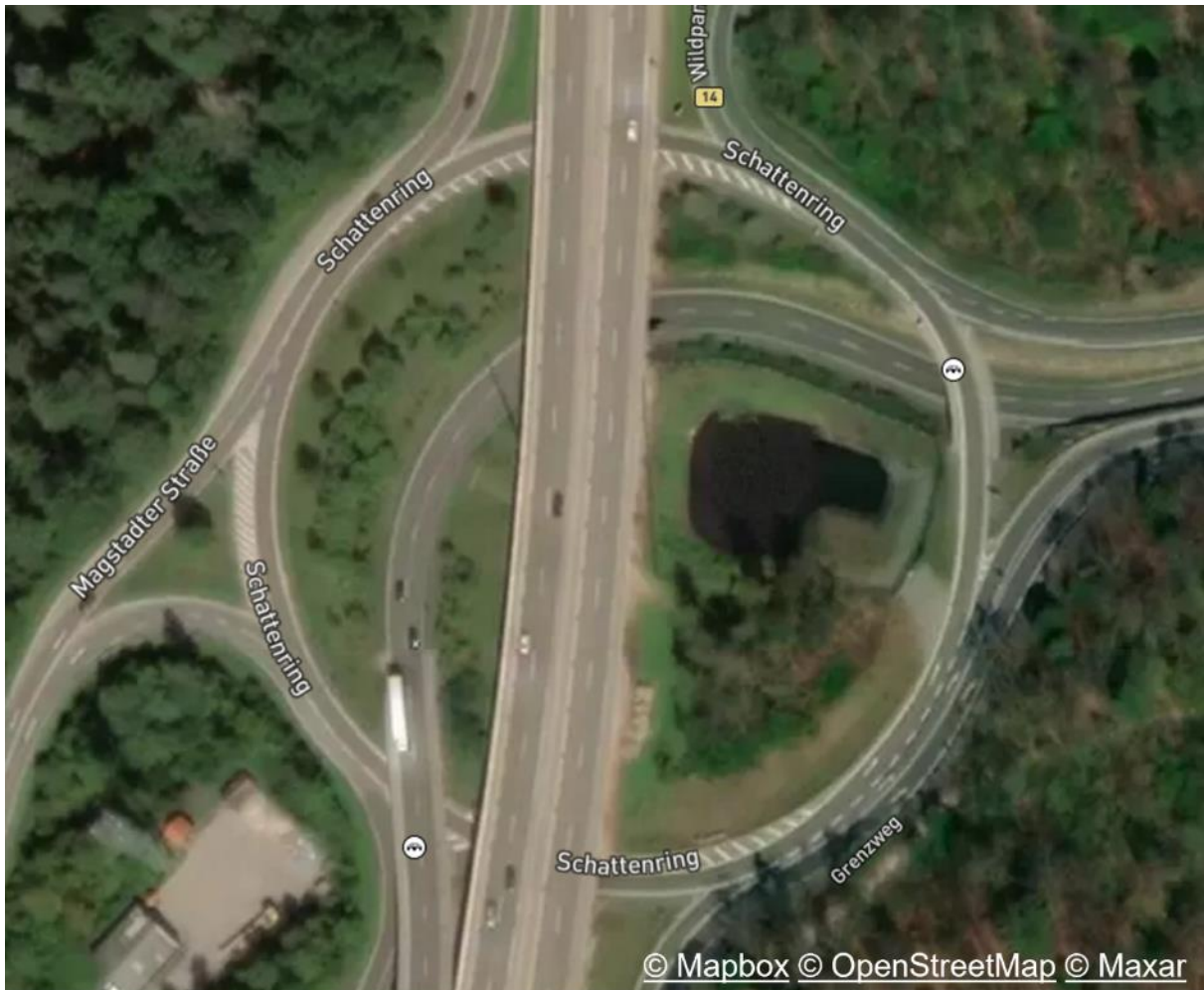
Figure 19: Roundabout with a non-constant number of lanes in a non-urban area. (Source: created using https://geojson.io © Mapbox (see: https://www.mapbox.com/about/maps/ ) © Maxar (see: https://www.maxar.com/ ))
