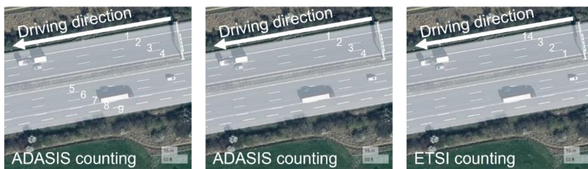
Figure 29: Example of the transformation algorithm, based on an imaginary ego vehicle within the segment. The white segment of this figure corresponds to the long blue segment in Figure 26. (Source: created using https://geojson.io © Mapbox (see: https://www.mapbox.com/about/maps/ ) © Maxar (see: https://www.maxar.com/ ))
