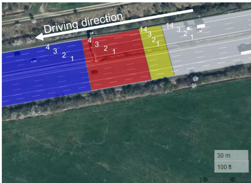
Figure 30: ADASIS-road segments for the scenario in clause 3.1 (where the exit lane starts) with the expected ETSI LanePositions. (Source: created using https://geojson.io © Mapbox (see: https://www.mapbox.com/about/maps/ ) © Maxar (see: https://www.maxar.com/ ))
