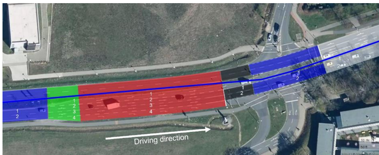
Figure 50: ADASIS-road segments for the scenario in clause 3.7 with the expected ETSI LanePositions for vehicles crossing the intersection straight. The solid line across the intersection is the more general path to follow. (Source: created using https://geojson.io © Mapbox (see: https://www.mapbox.com/about/maps/ ) © Maxar (see: https://www.maxar.com/ ))
