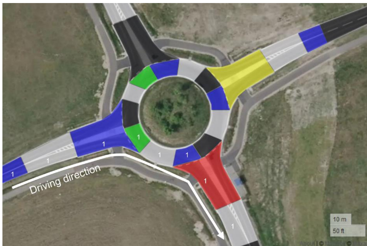
Figure 54: ADASIS-road segments for the scenario in clause 3.9 with the expected ETSI LanePositions . (Source: created using https://geojson.io © Mapbox (see: https://www.mapbox.com/about/maps/ ) © Maxar (see: https://www.maxar.com/ ))
