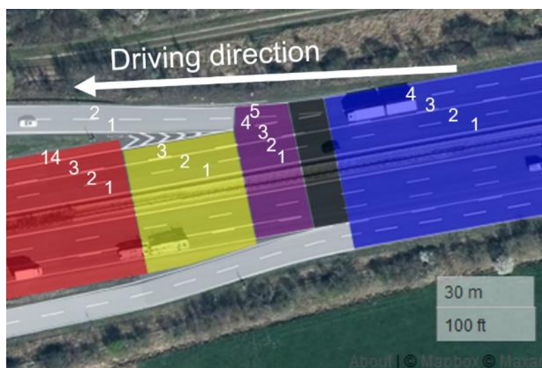
Figure 31: ADASIS-road segments for the scenario in clause 3.1 (where the second exit lane starts) with the expected ETSI LanePositions. The purple and grey segment use the same lane numbering, but it is not shown for the grey segment due to readability. (Source: created using https://geojson.io © Mapbox (see: https://www.mapbox.com/about/maps/ ) © Maxar (see: https://www.maxar.com/ ))
